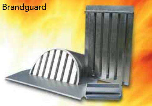
The "Vulcan Vent®" (left) is one of three vent systems approved by the California State Fire Marshal for use in building construction in the WUI. The other approved vents at the time of printing are "Brandguard®" (middle) and "Embers Out®" (right). Available in different sizes and applications, these vents reduce ember entry and can seal the opening off when exposed to flames and/or radiant heat. O'Hagin Fire & Ice® Line – Flame and Ember Resistant Vents (not pictured) are a good option for through roof vents.
