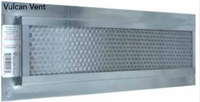
The "Vulcan Vent®" (left) is one of three vent systems approved by the California State Fire Marshal for use in building construction in the WUI. The other approved vents at the time of printing are "Brandguard®" (middle) and "Embers Out®" (right). Available in different sizes and applications, these vents reduce ember entry and can seal the opening off when exposed to flames and/or radiant heat. O'Hagin Fire & Ice® Line – Flame and Ember Resistant Vents (not pictured) are a good option for through roof vents.
