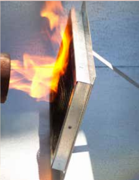
Commercial vents are available that resist both ember and flame entry, while allowing proper ventilation (photo courtesy of Vulcan Technologies).
